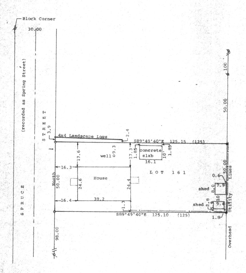
Scale - 1' - 20'  $\emptyset = 3/4$ " Iron Pipe Found Q = 14" Iron Pipe Found • = 1 x 24 Iron Pipe Set 0 = 3/4" X 24" Iron Pipe Set (0.00) = recorded distance Bearings referenced to the assumed bearing of North along the east line of Spruce Street Survey ordered by: Realty World, Carmin Realtors 811 East Geneva Street Delavan, WI 53115 ----- fence line
